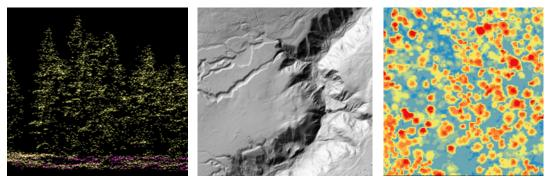
*Figure 5. Example data acquisition products from LiDAR: a) Point cloud-profile view; b) Hillshade – plan view; c) Canopy height – plan view.*
