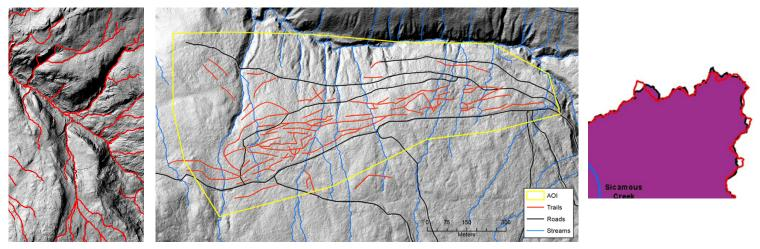
Figure 6. Mapping of streamflow paths (left), watershed boundaries (right), and legacy roads and trails (centre) using LiDAR.
