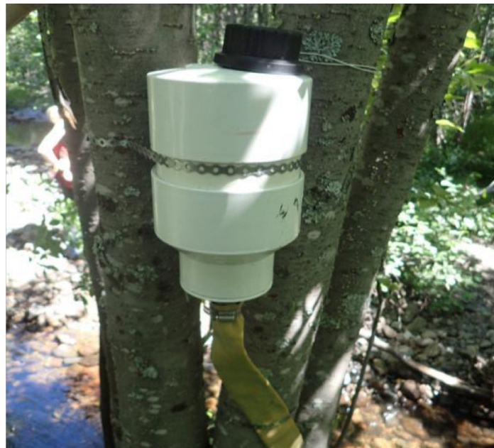
Figure 2: Example of direct read setup with cable protected by fire hose buried in a stream channel during low flows. Set-up provides terrestrial access to retrieve logger data at all flow levels (Image: Chelton van Geloven).
