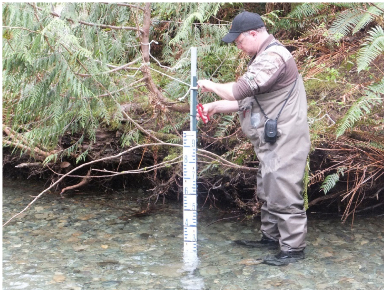
Figure 1. Example of a temporary, low-flow hydrometric station. A non-vented pressure transducer is housed in a PVC stilling well with an external staff gauge that is tethered to the streambank. The equipment is anchored and levelled during install using T-bar and a modified cement paver. This type of station is not meant for long-term or high-flow applications and typically will only be used for a few months in the summer (Image: Dave Spittlehouse).
