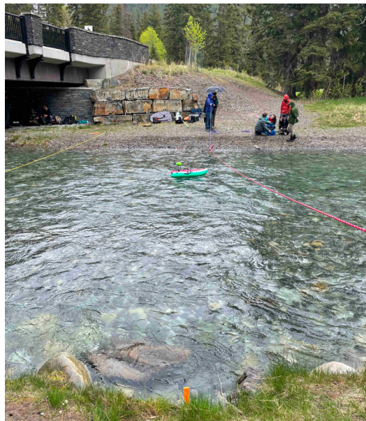
Figure 1. Measurement of streamflow at Spray River near Banff during the 2022 regatta by an Acoustic Current Profiler (ADCP) (left panel) and an Acoustic Velocimeter (ADV) mounted on a wading rod (right panel). Photo credit: Derek Brzoza
